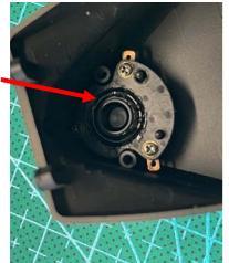
**2.** Apply glue as indicated. Adjust the spirit so that the bubble is on the center.
