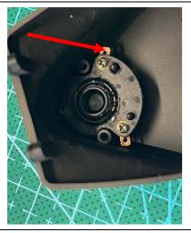
1. We recommend to put back the spacers and secure the screws as original.
