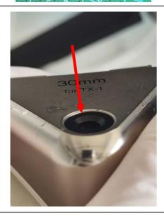
3. Assemble the upper and lower viewfinder case. Secure the viewfinder on a leveled camera, adjust the level from upper. You may find the spare part surface is not parallel with the surface of upper case, it is NORMAL. Picture on left is viewfinder from Fujifilm. The level spirit is slightly angled.
